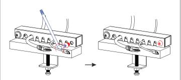
2A - Using included specialty tool, completely remove one of the horizontal, front facing screws. Open the cable holder component as shown. Place all the desired cables to be secured and organized in between the grooves. Close the top component and place back original screw with included tool until securely tightened.
