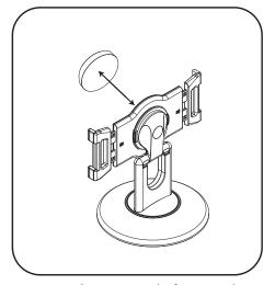
Optional: Use a single foam pad to fill the space between tablet and holder for tighter fit and grip.
