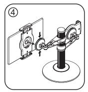
Squeeze buttons on either side of attachment arm, attach bracket and rotate until you hear a click.
