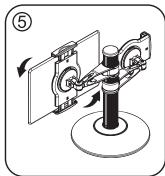
Tablet can safely be rotated 360 degrees.
