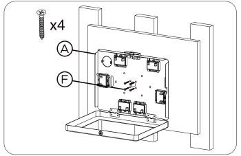
6A. Hold enclosure at the desired mounting location. Rotate in screws (F) with screwdriver tool (not included) until securely tightened.
