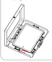
1C. Plug in the charging cable (not included) and route the cable out the back hole as illustrated.
