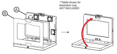
4A. Lay-in correct masking insert from bundle (B) as needed for the correct setup for your device.
