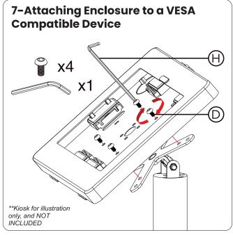
7A. Align enclosure holes to VESA plate holes. Rotate the screws (D) above using provided allen key tool (H) until securely tightened.
