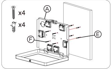
5A. Insert the (4) wall plugs (E) to the wall pre-drilled holes. Then, align VESA holes as shown above to the drilled holes and screw in the (4) screws (F) using a screwdriver tool (not included) until securely tightened.
