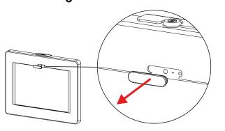
3A. Remove the cover as illustrated to use tablet with front camera exposed as needed.
