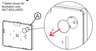
2A. When installing device into the enclosure, identify where the camera is. Then simply remove and pop out the cover prior to mounting or setting up tablet to properly expose camera.
