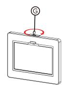
4B. Once the tablet device is set up, close the front lid of the enclosure. Insert the key (G) in the keyhole at the edge of the enclosure. Rotate and lock it in place.
