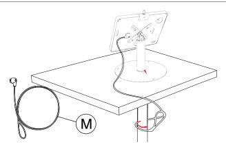
4A. Take the looped end of lock cable (D) and turn it around leg table then click-in head of lock cable into the security hub.
