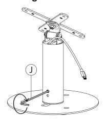
Turn clockwise to prevent body rotation using the provided allen key tool (J).
