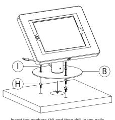
Insert the anchors (H) and then drill in the nails (I) to the mounting surface as shown above.
