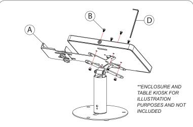
2A. To setup, align VESA holes of a compatible CTA Digital enclosure and base mount or any other similar compatible items - with the Card Reader Holder VESA holes. Rotate in screws (B) from above using provided tool (D) while holding hex nuts (C) from behind using your hands as illustrated. Rotate until securely fastened.
