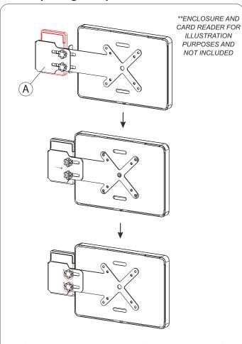
3A. Slide the loosened card reader holder to fit the card reader device. Once you have a tight and secure fit, rotate the knobs on the back until securely tightened. Your setup is now complete.
